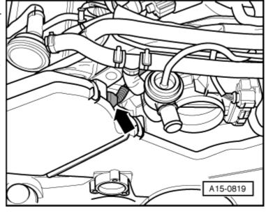
Disconnect the camshaft adjustment solenoid valve connector -1-.
